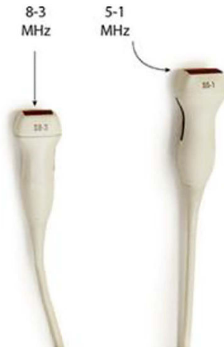
Figure 2. High-frequency phased array probes used in focused cardiac ultrasound (FOCUS; figure courtesy of Vrushali Ponde).
